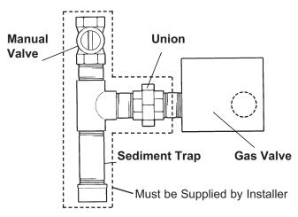
Fig. 14: Sediment Trap
